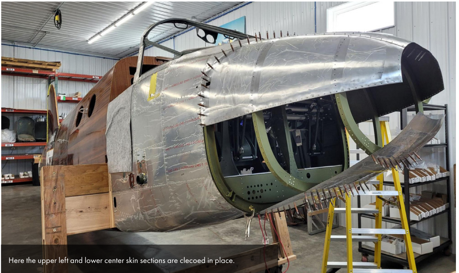
Aaron has begun assembling the demountable nose frame and skin sections.
