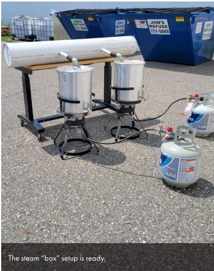
Aaron had to make a steam apparatus to form a curve in the forward spar. This plastic pipe was the starting point.
