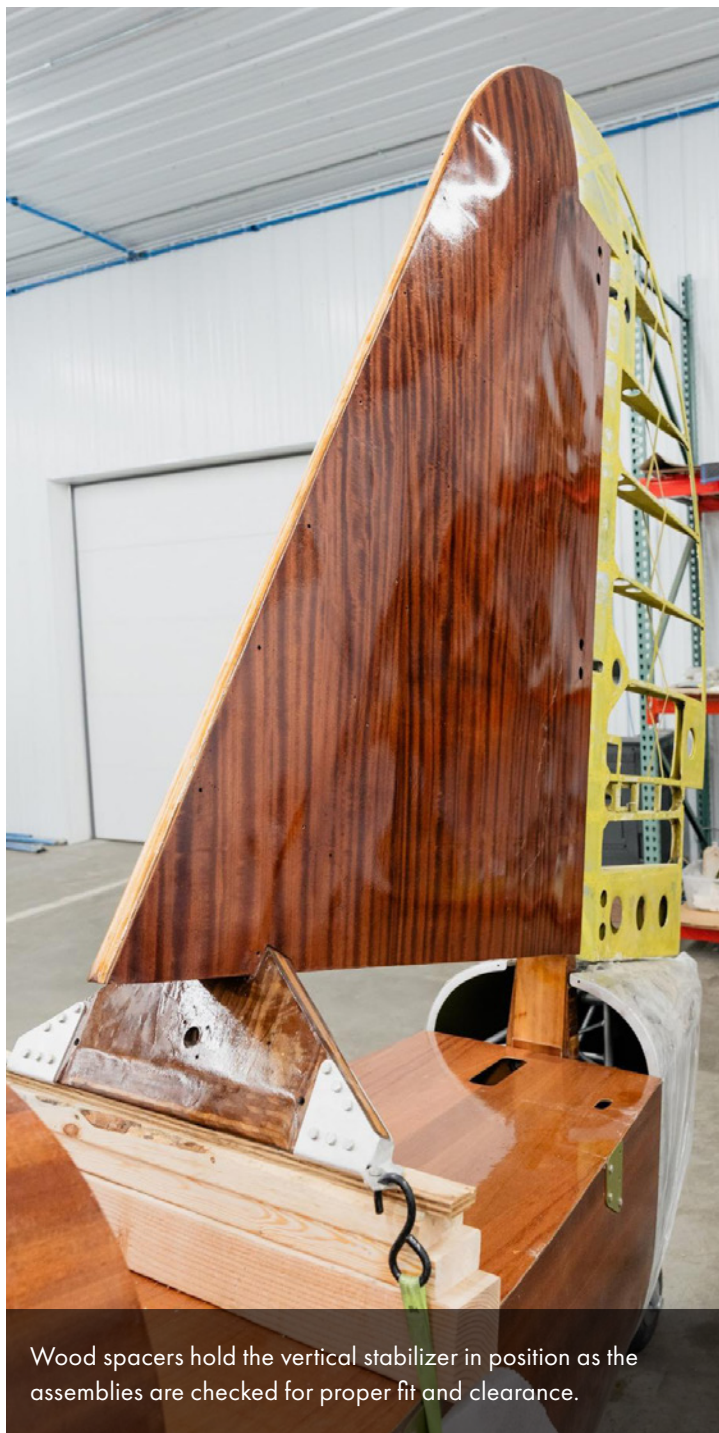
The rudder was found at a tech school and is in good condition, for an 80-year-old assembly. However, it will require restoration work on some ribs and the leading edge.
