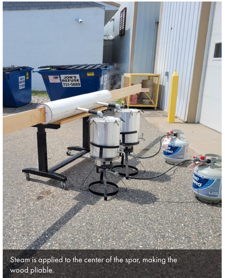
Aaron had to make a steam apparatus to form a curve in the forward spar. This plastic pipe was the starting point.
