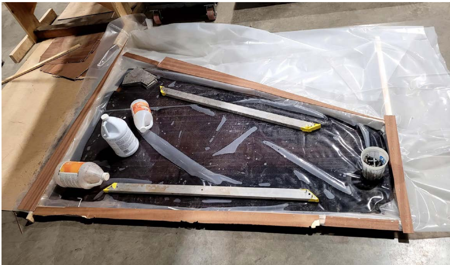
A skin section is soaked in ammonia and water to make it bendable for forming over curved sections.
