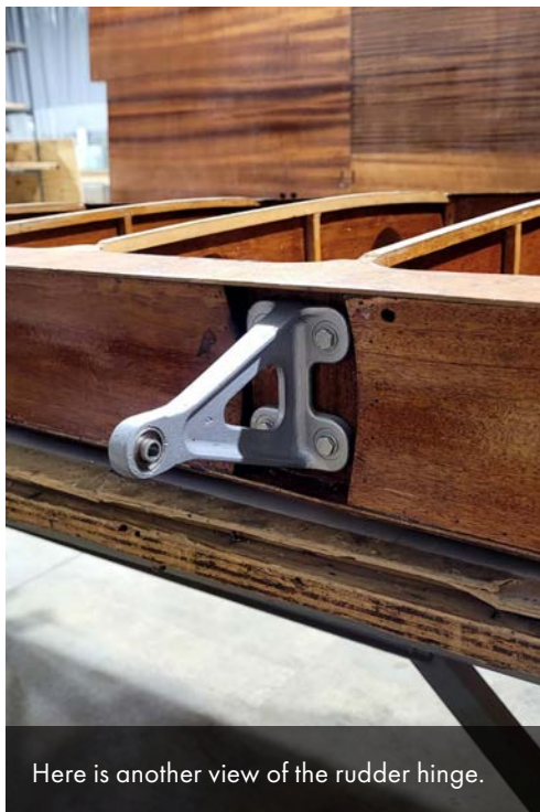
The edges of the ribs and all gluing surfaces have been carefully sanded.
