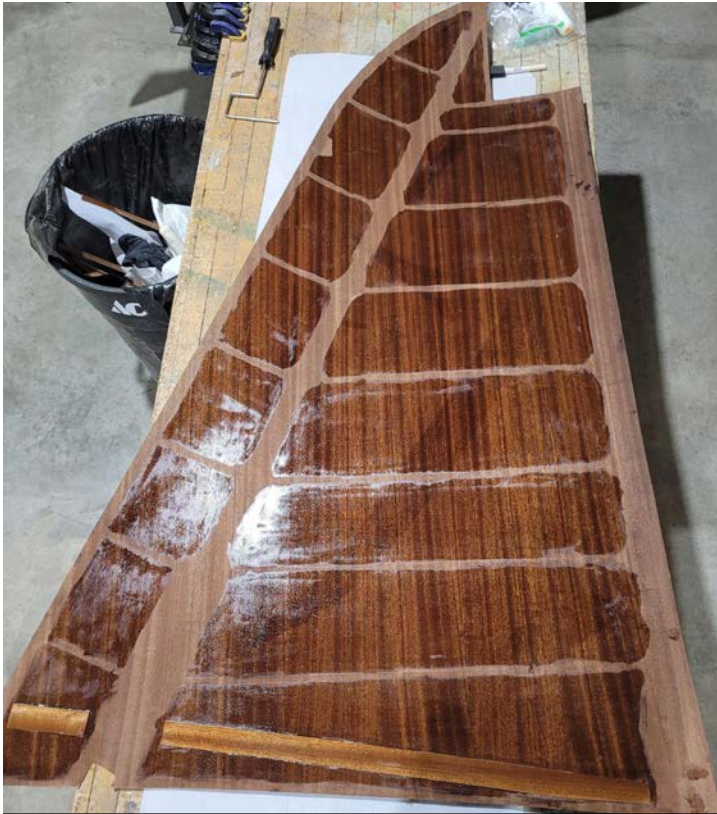
Epoxy coats the areas of the skin that will not have glue applied.
