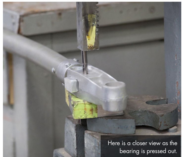
Lance presses out an old bearing from the P-47 control stick.
