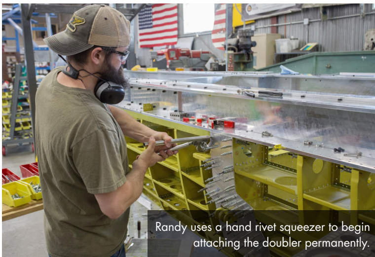
The first few rivets are visible at the top of the doubler.
