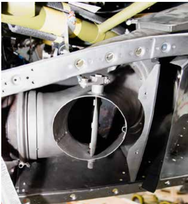
The waste gate shown here is in the position that would bypass the turbosupercharger system. It opens and closes to regulate the exhaust gas pressure to the turbosupercharger. It's purpose is to control maximum boost.
