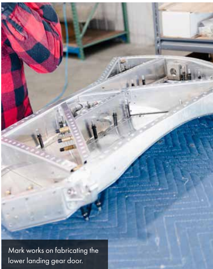
It takes many clecos to hold everything on the landing gear doors in alignment as holes are drilled and rivets set.
