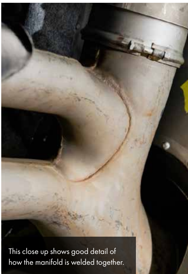
The right side manifold section shown here exits into a duct leading to the waste gate and on to the turbosupercharger.
