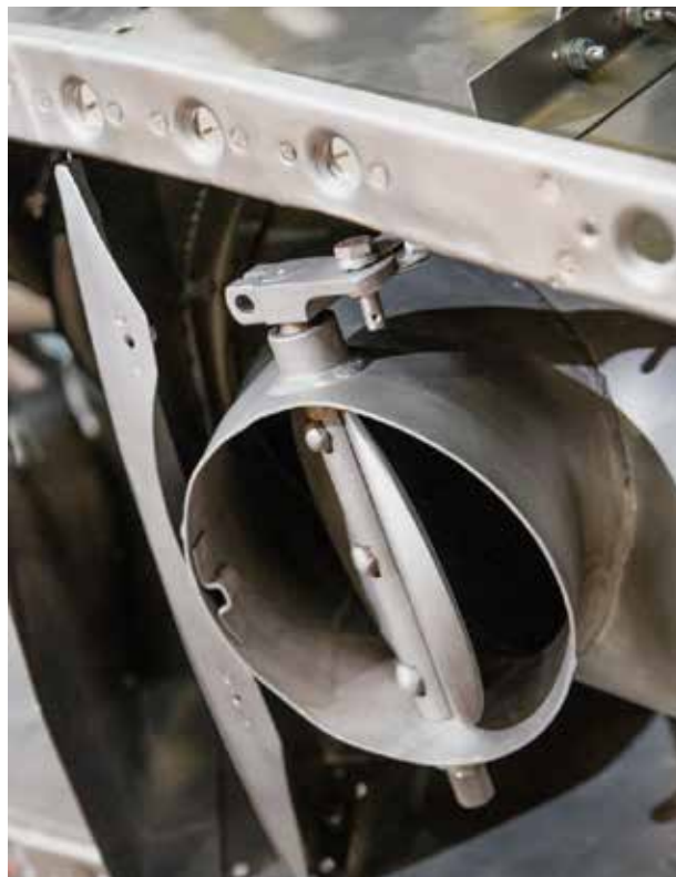
Here is a close up of the waste gate partially closed.
