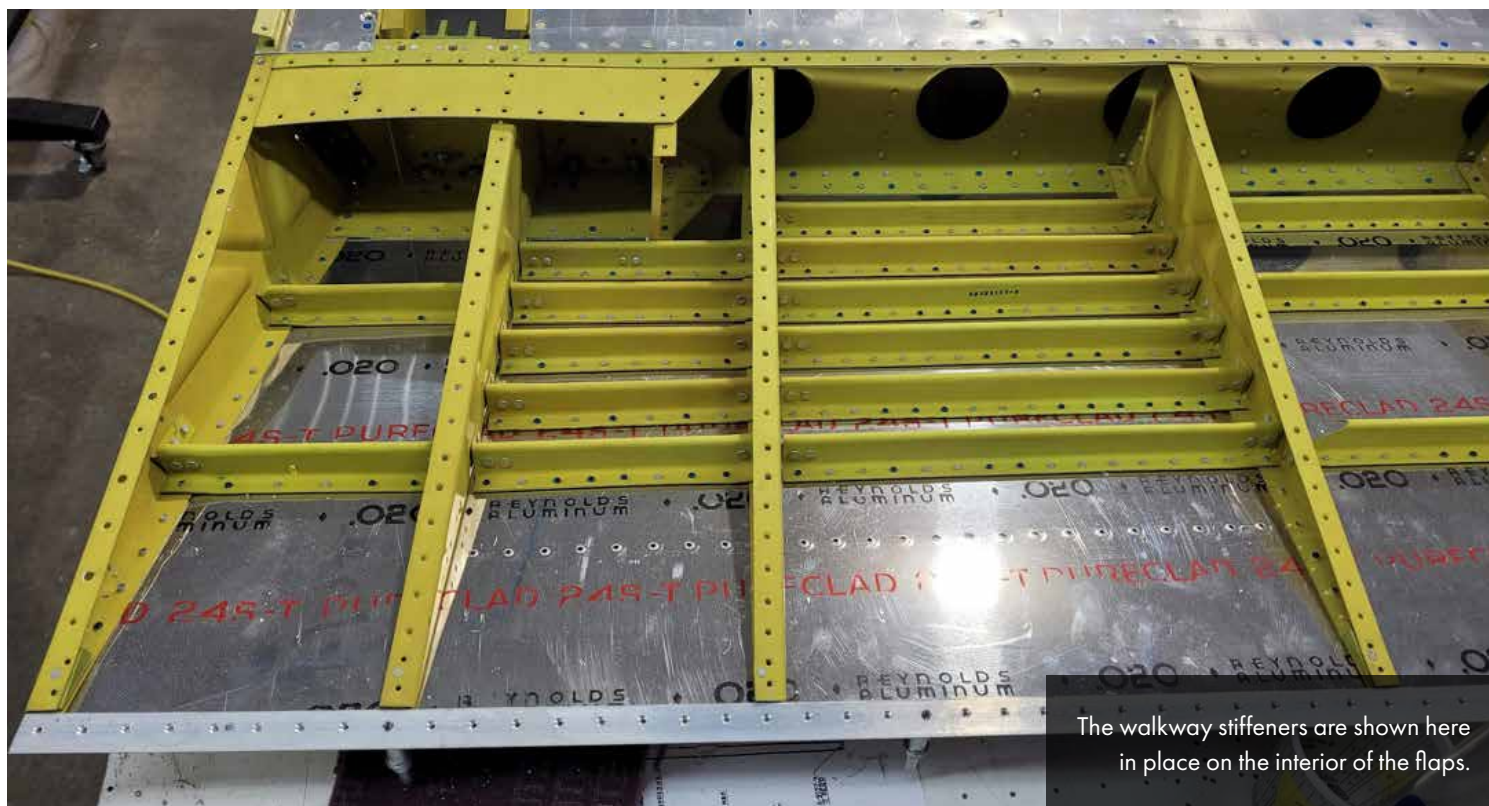
Cory prepares stiffeners that support the walkway on the flaps.
