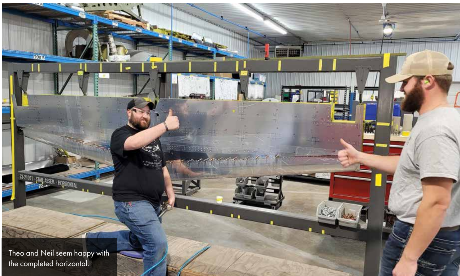
After the painting was completed, the horizontal stabilizer had its skins riveted on.
