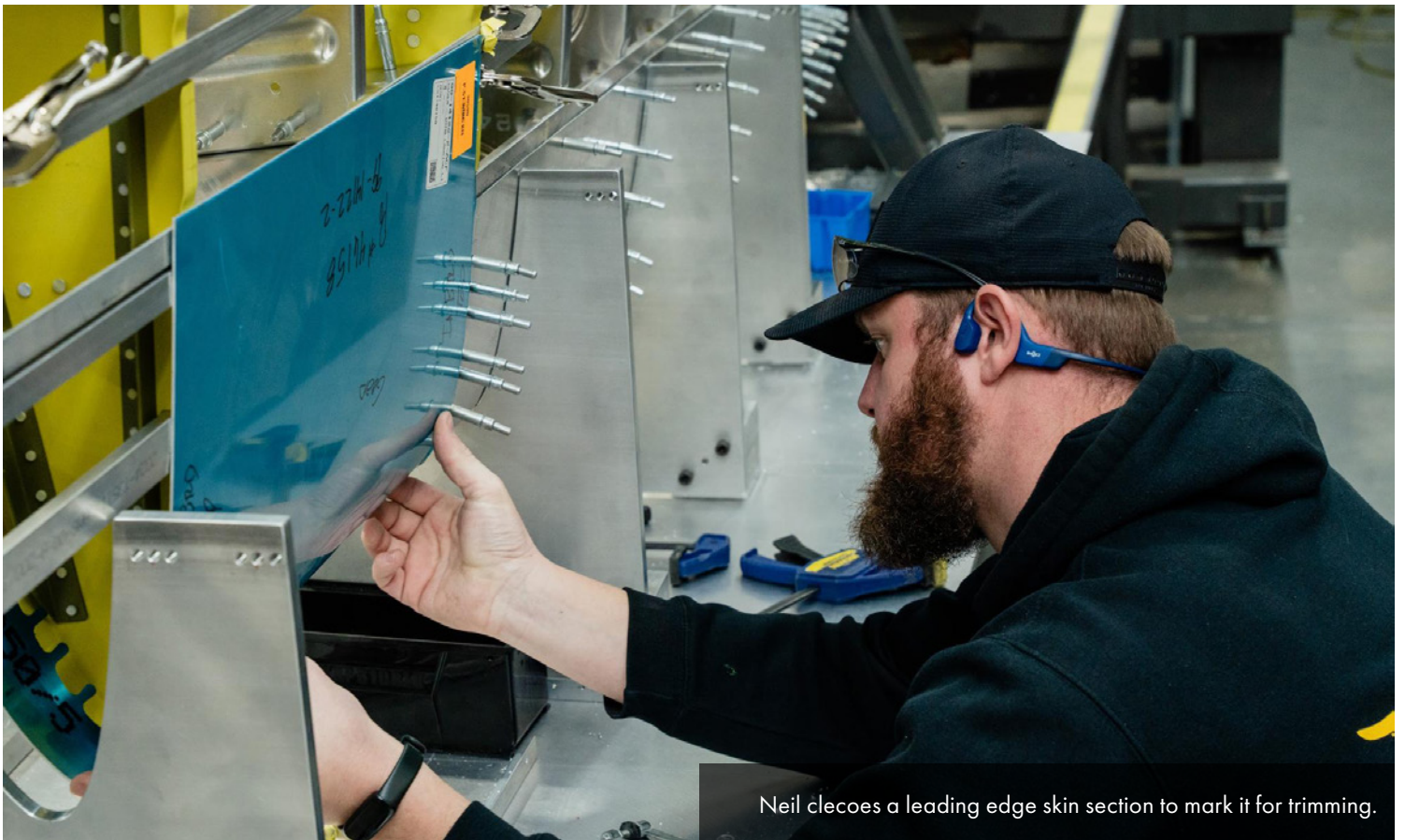
Zach looks intent as he installs some clecoes on a new section of wingskin.
