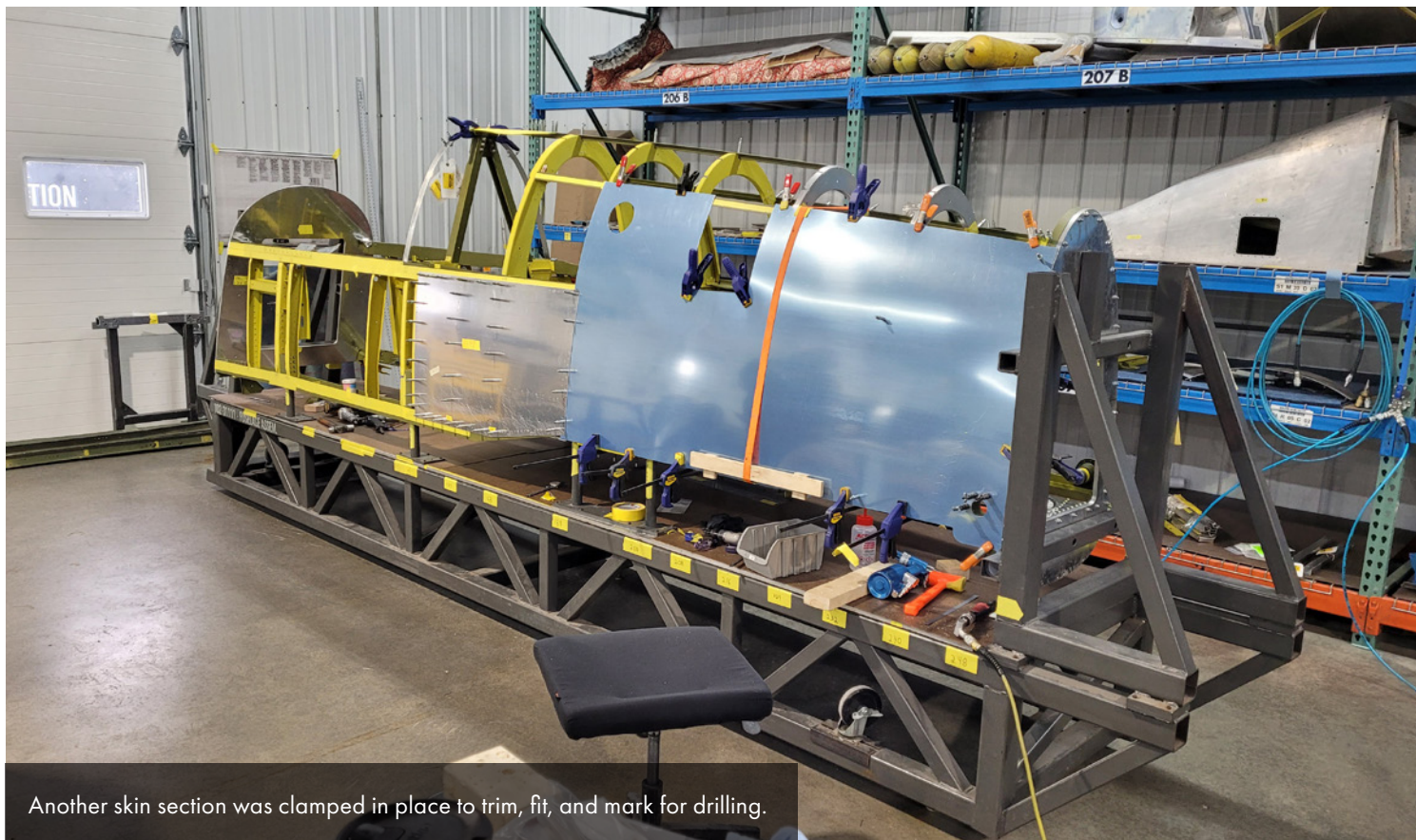
One by one skin sections are cut, drilled, deburred, and fitted into place
