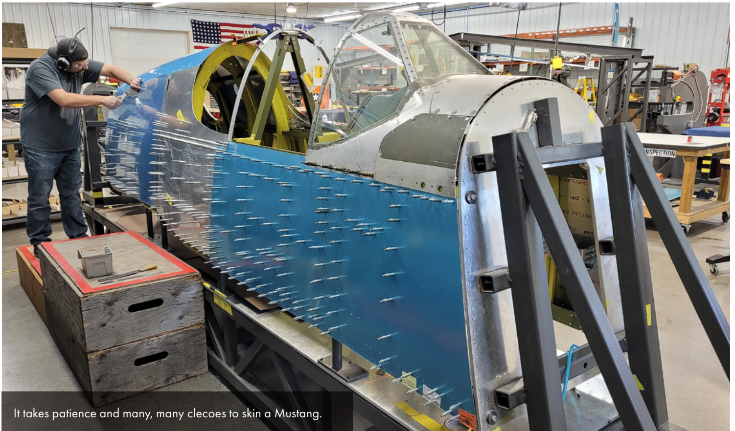
The top turtle deck skin has been stretch-formed and the edge slid under the side skins to mark where it needs to be trimmed.
