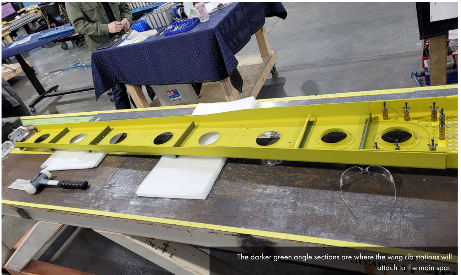
The main spar has been painted and returned to the restoration shop.
