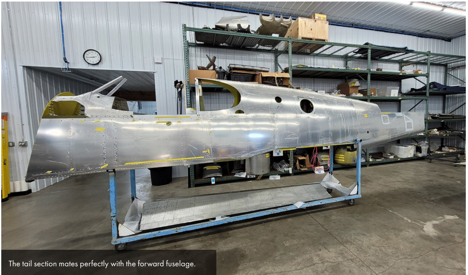
After the riveting of the skins was completed, the fuselage was mounted on a movable fixture.
