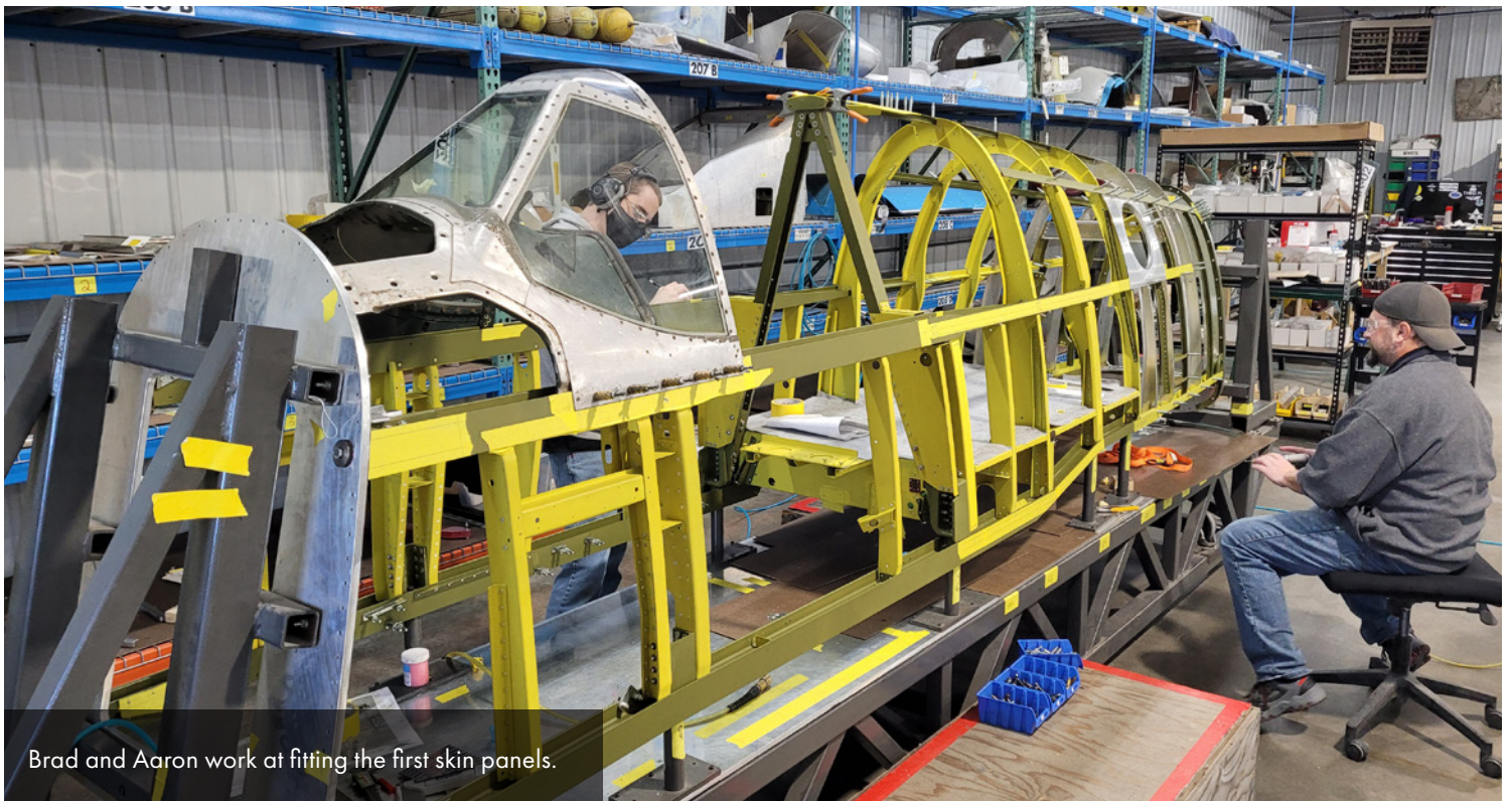
The fuselage components have returned from the paint shop and the windshield has been mounted.
