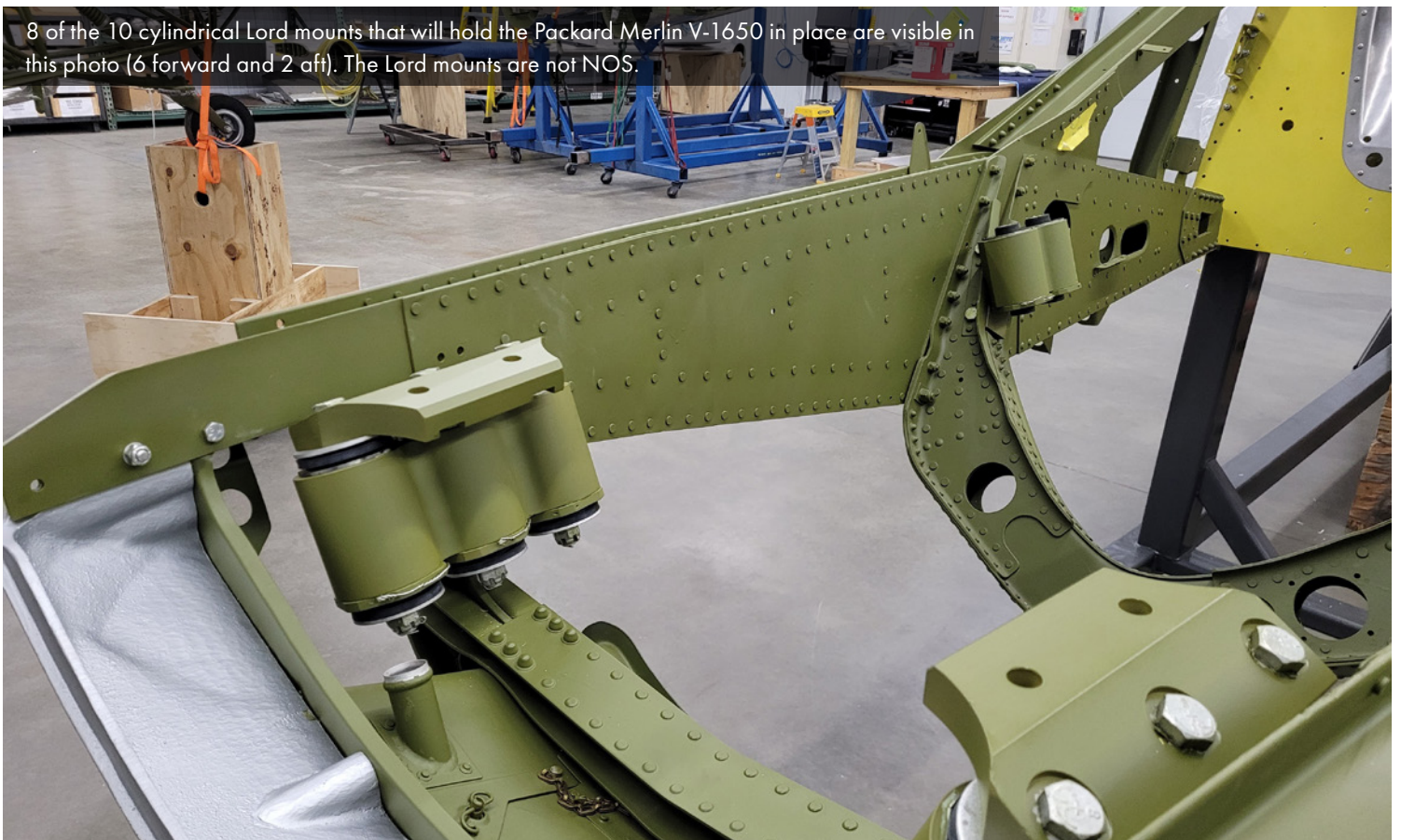
The engine mount is one of the NOS assemblies used for the Shillelagh restoration. Despite being built in the 1940s, it has never been installed in a Mustang and has its original hardware.
