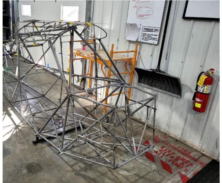
The repaired and straightened frame as it was returned to AirCorps.
