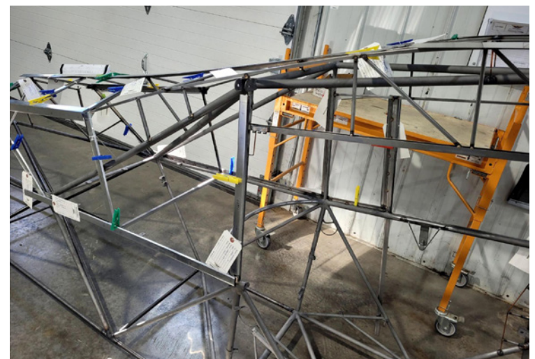
The rear window area shows one of the main structural differences between an L-4 and a J-3.
