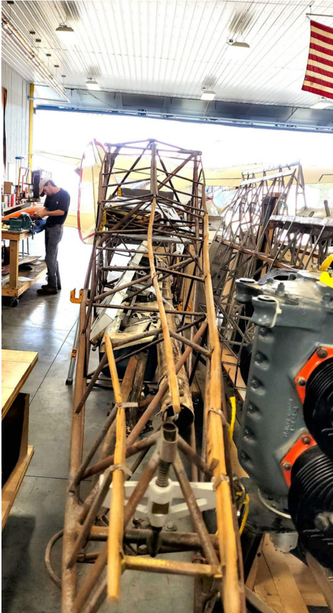
The damaged fuselage frame at the start of the project.
