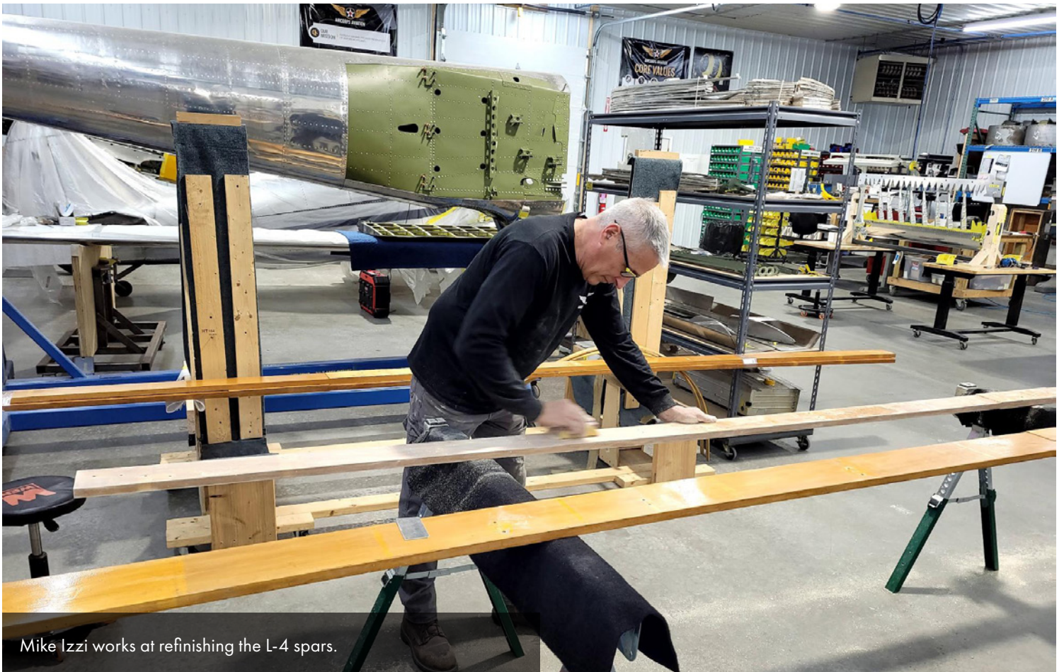
The wings have been disassembled and the spars inspected. They needed refinishing but were otherwise airworthy.
