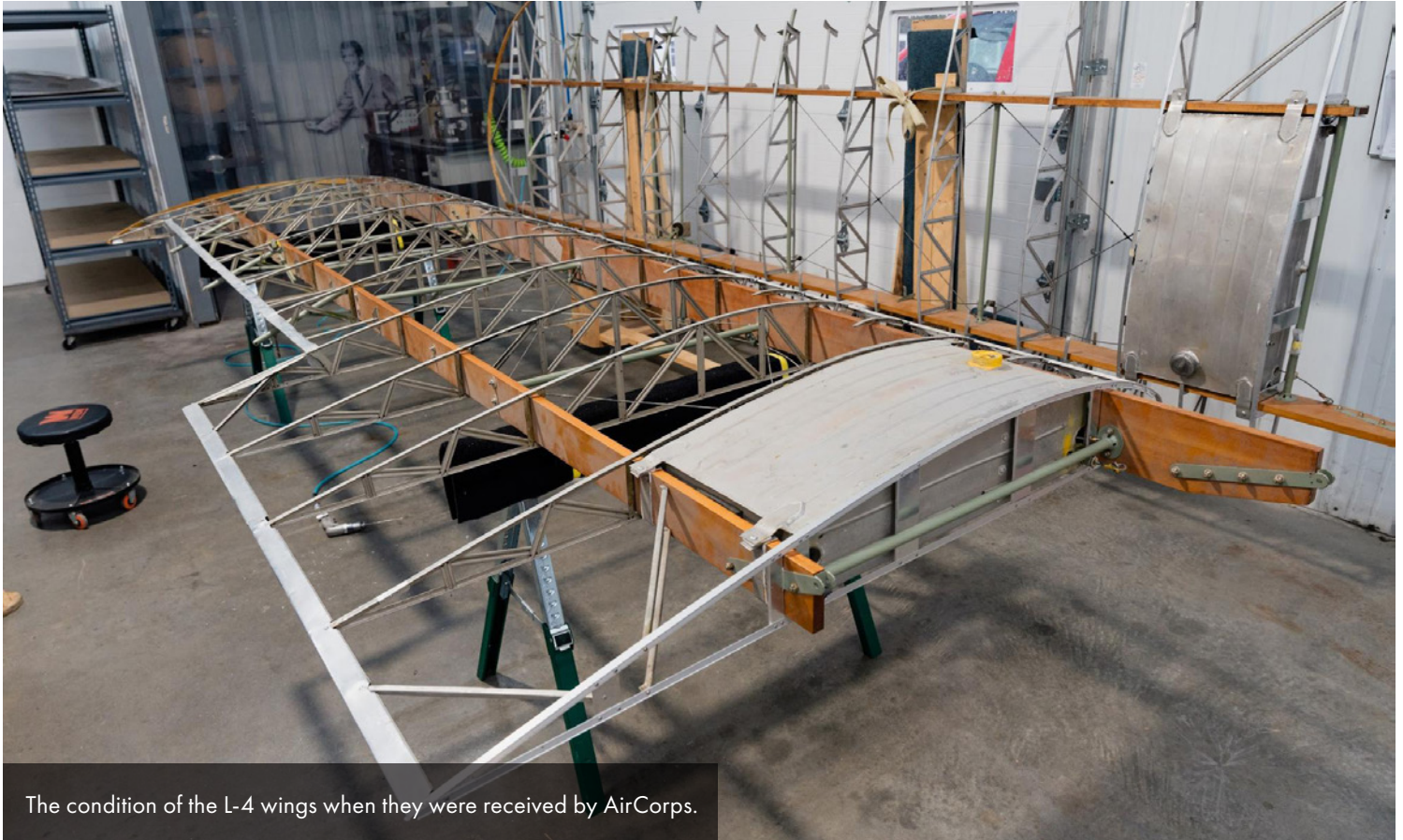
There were many past repairs, especially to the ribs.
