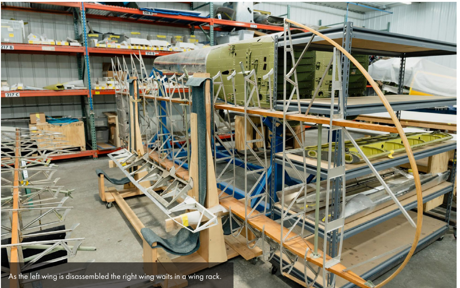
A view from the tip of the left wing as disassembly progresses.
