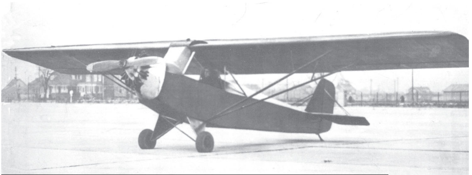
Taylor E-2 Cub with the Salmson engine that replaced the unsuccessful Tiger Kitten. W.Finch Jr collection 2
